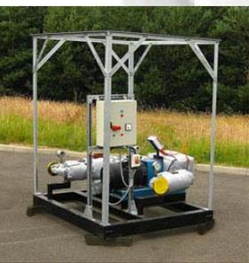
Demand for a standard loading/unloading system for Bitutainers™ has led TEC to develop these complete, skid mounted pumping systems with electric cartridge heating, insulation and control panels.
